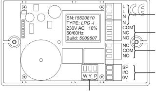
Power Supply With Auxiliary Output Terminals
